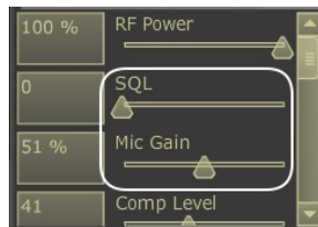
Set Squelch to 0 for HF, Mic Gain at the center
