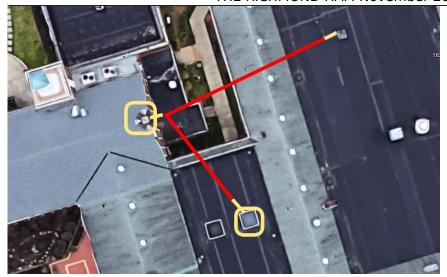
The HF antenna is a 95ft end fed long wire installed in a "L" configuration from the sky light over the commons area of the church to the chimney / ladder over the kitchen and across the courtyard to the gym roof.
