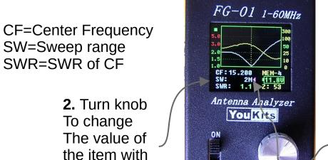
the red arrow MEM=saved CF,SW Green digits=battery voltage Z: Impedance at CF
