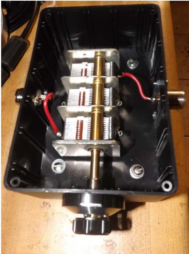
Contrary to conventional wisdom, the center and shell of the SO-239 connectors are shorted with grounding lugs. This is because both the shield and inner conductor of the LMR-400 cable are tied together to form the large loop.
