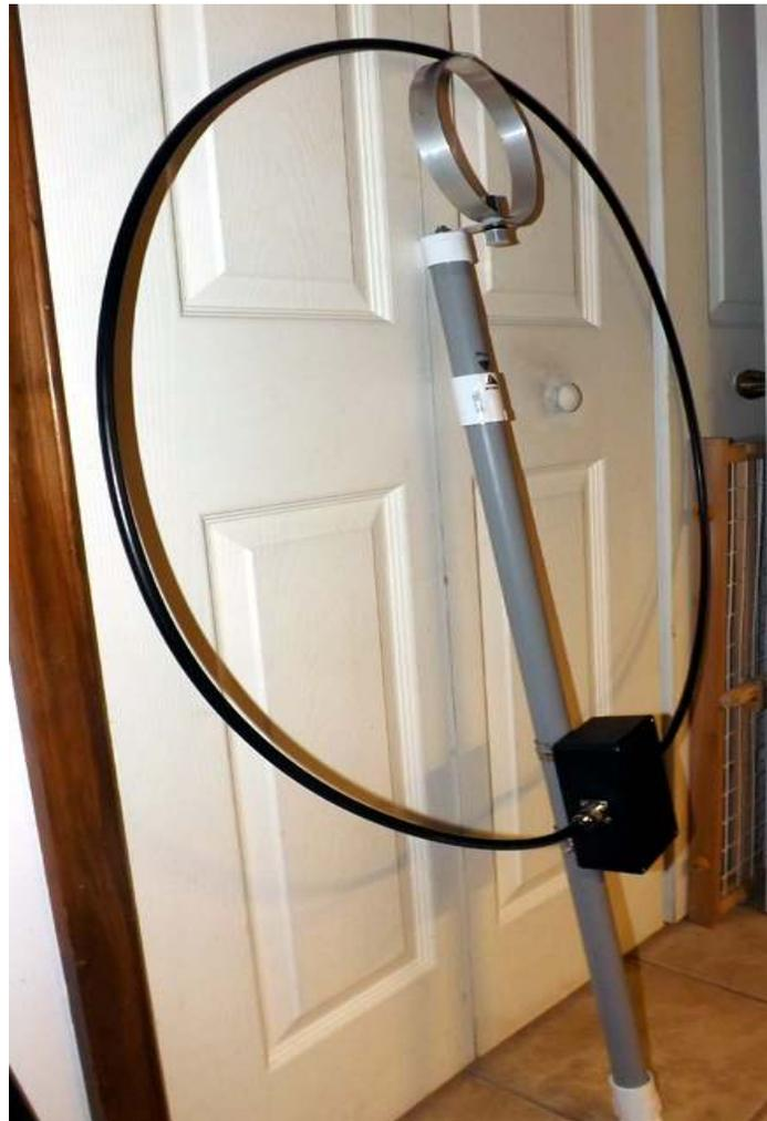
Now cut the top section of the mast to the proper height and install the Faraday loop assembly so that the top of the Faraday loop is even with the top of the main loop. Wrap the velcro to hold the tops of the two loops together.
