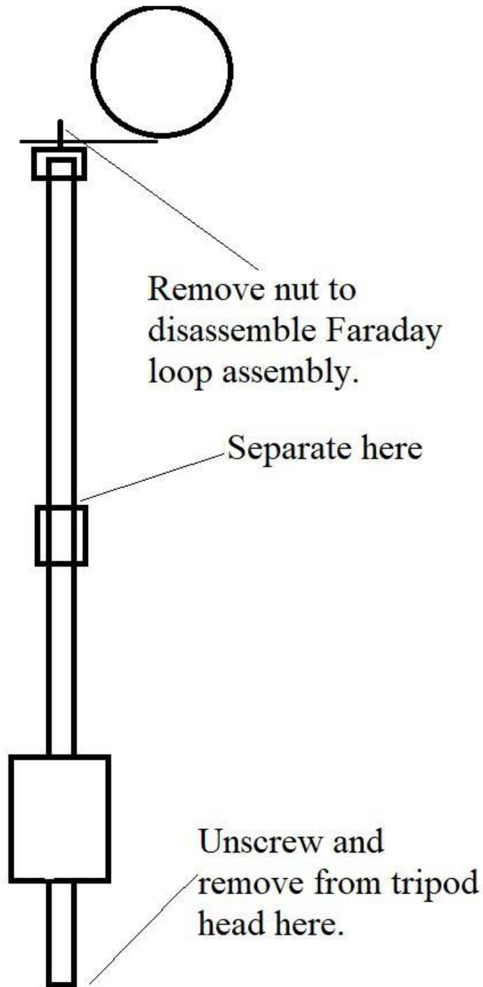
The antenna breaks down into 6 sections for storage or transporting:
