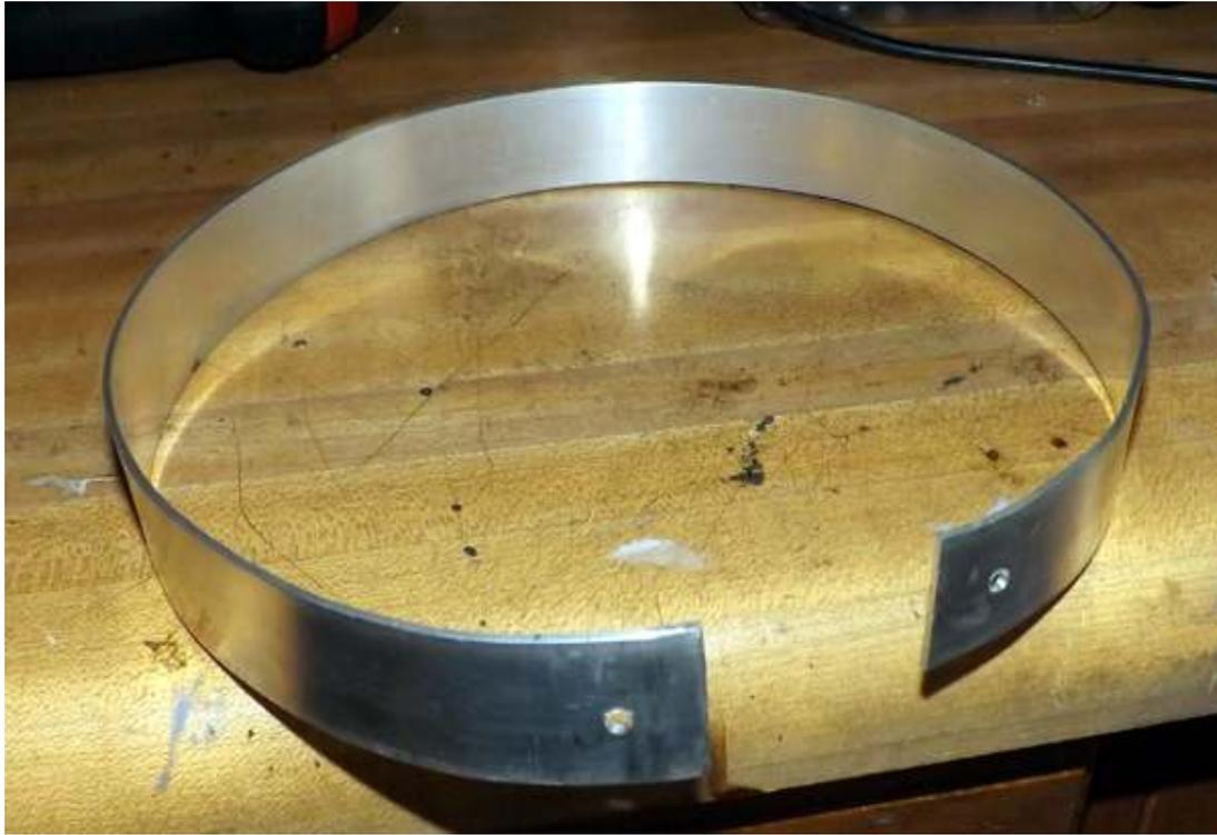
We started by cutting a piece of the 1" aluminum flat bar to a length of 23".
