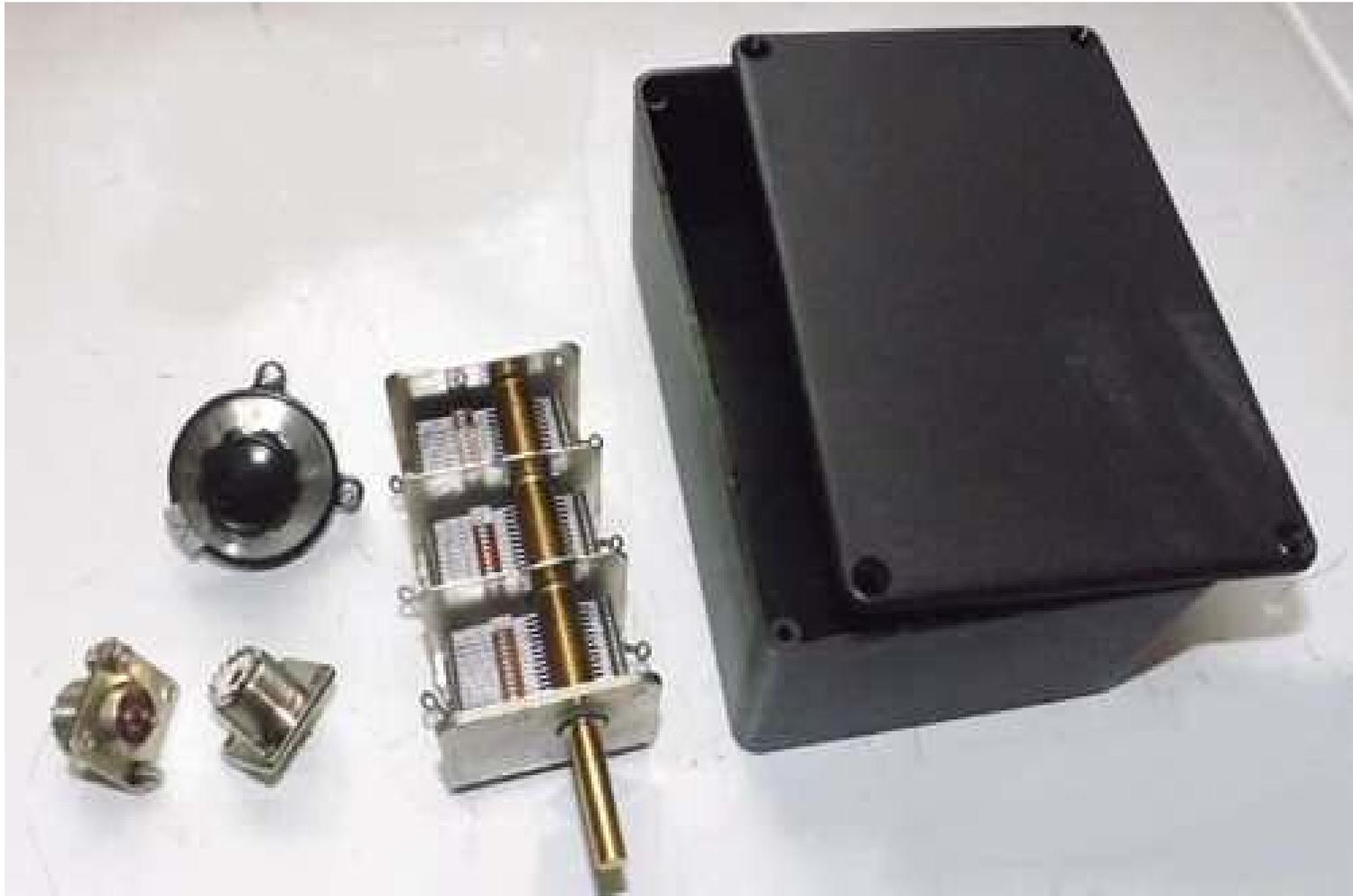
This is how the tuner enclosure is prepared. It is helpful to make a template of the bottom of the capacitor for drilling accurate holes.
