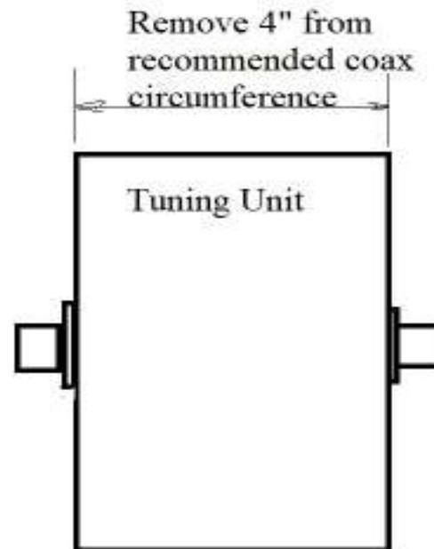
Cut coax to 96.79" before connector installation.
