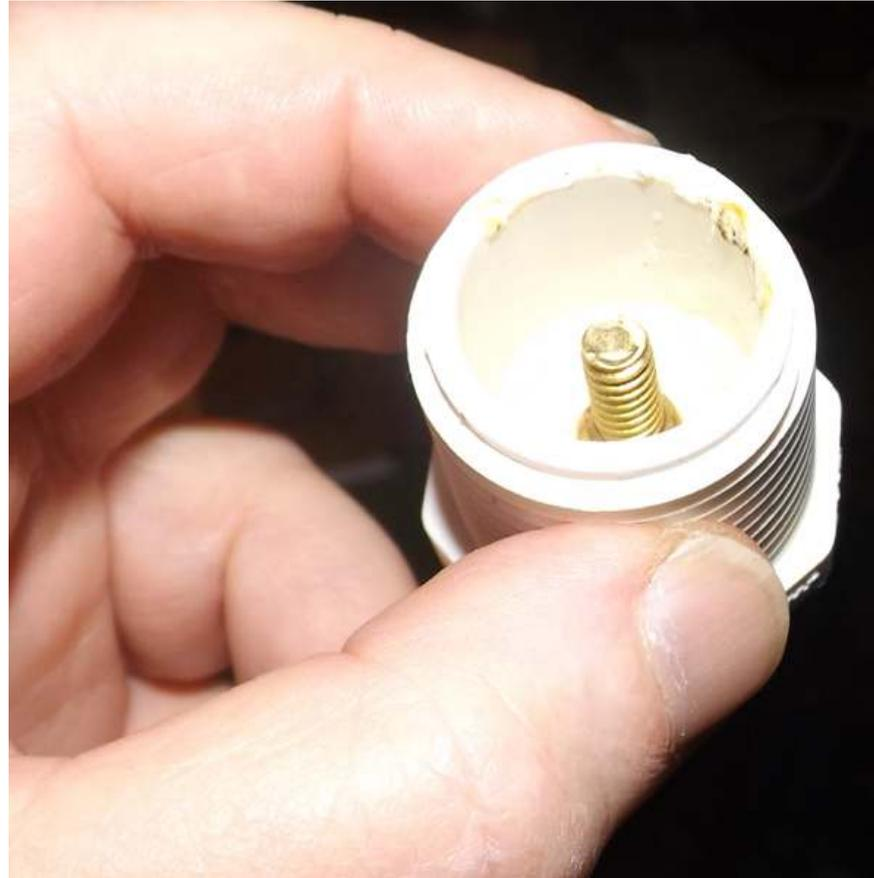
The bolt shown in the insert is temporary to insure alignment of the brass insert. Epoxy glue has been poured into the cap to a level just below the top of the brass insert. The brass screw can be covered with a thin layer grease to insure that it can be removed in the event that any glue leaks onto the threads.
