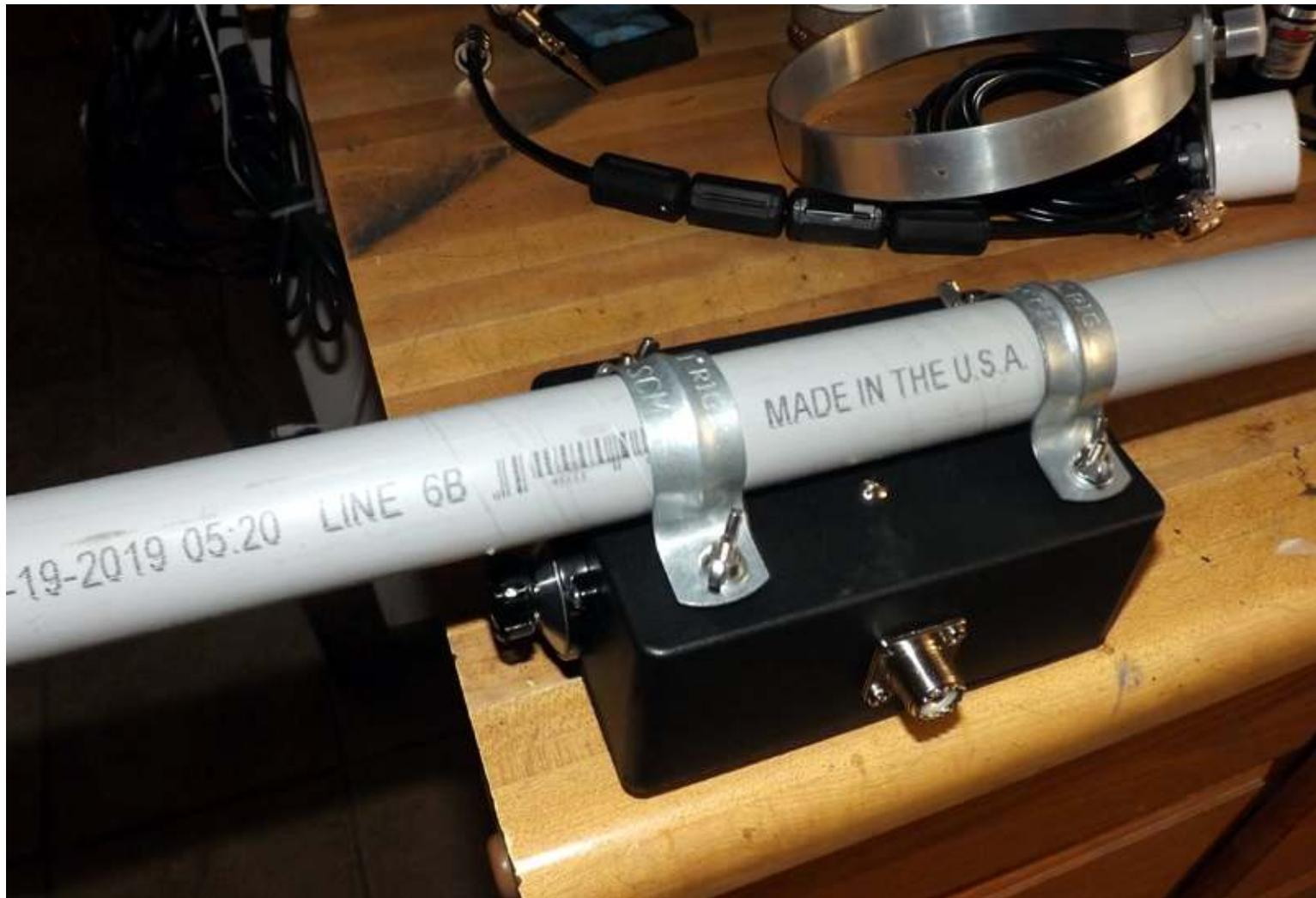
After measuring and cutting the LMR-400, and installing the connectors, the cable can be attached to the tuner in preparation for measuring the remaining section of the mast.
